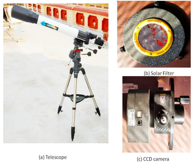
Fig. 3. Experimental facilities for solar measurements: (a) Telescope, (b) Solar Filter and (c) CCD camera.
