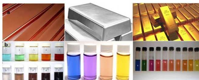
Fig. 8. Coinage metal (Cu, Ag & Au) in their bulk state (a) and at nanoscale level (b) showing different colors
