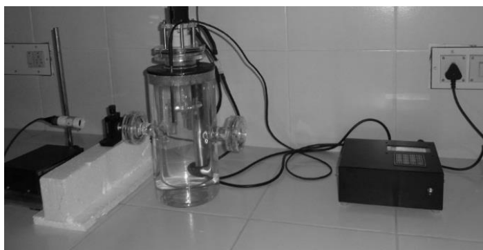
Fig.1. Crystallizer with stepper motor and PID based temperature controller
