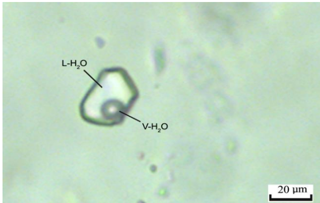
Fig. 2. Photomicrograph of quartz showing aqueous Biphas subrounded isolated Fluid Inclusion at room temperature. SK mine of Rajpura-Dariba-Bethumni Belt, Rajasthan.
