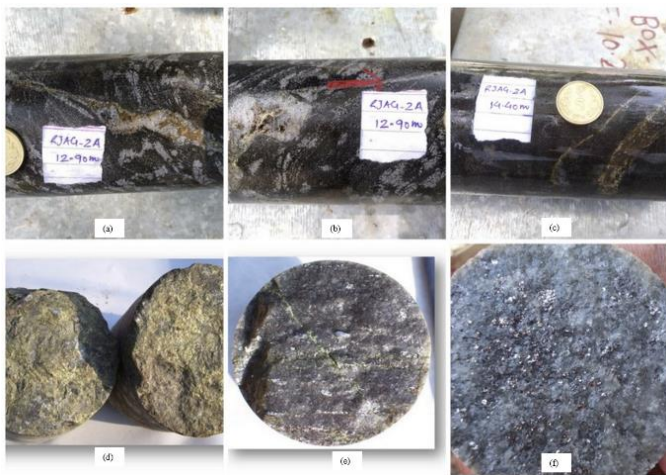
Fig. 13 Core Sample of different rock type from variable depths (a-c) showing Chalcopyrite (greenish yellow) and Pyrrhotite (bronze red) mineralization in the form of veins, stringers and foliation parallel (d) Chalcopyrite mineralization (greenish yellow) in massive from (e) Arsenopyrite (silvery white) and Chalcopyrite (greenish yellow) in Dissemination form (f) Arsenopyrite mineralization in dissemination.
