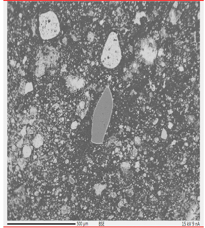
Fig.5: Photomicrograph showing magnetite (light) and chromite (gray) in dark silicate matrix (PPRL)
