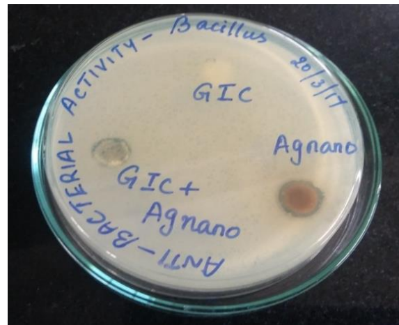
Fig. 12. Anti-bacterial Activity of Silver Nano Dental Composite I (5mg of AgNP with 2:2 ratio of powder and liquid) against Bacillus cereus
