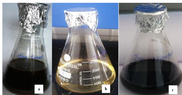
(a) Aqueous clove extract (b) Ferric chloride solution (c) Iron nanoparticles
