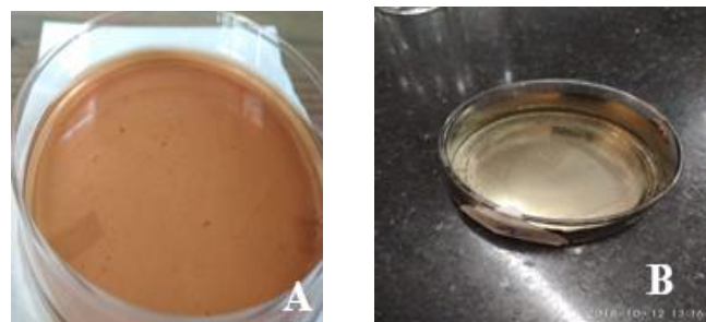
Fig. 3: Collection of purified and concentrated AgNPs sample synthesized from the combination of leaf extracts; (A) The purified AgNPs pellets were decanted in a petri dish after removal of contamination, (B) The concentrated AgNPs obtained after oven drying the pellets for 24 h.
