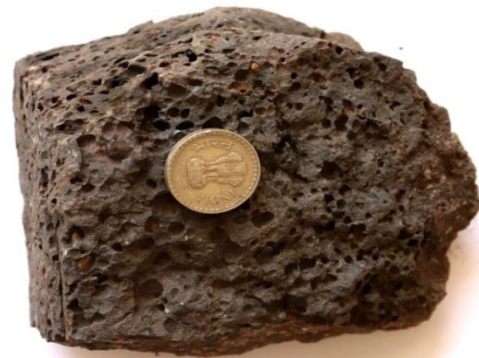
Fig. 4: Sample of Basalt showing the vesicular nature
