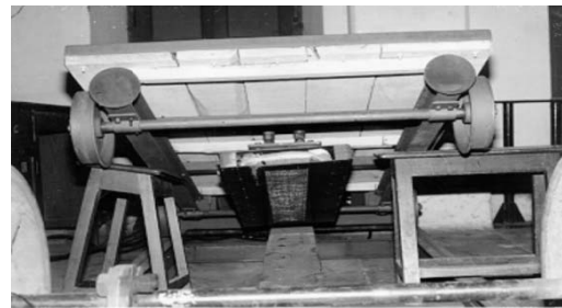
Fig 5 Trolley with LIM Primary lifted-up to show the underside arrangement
