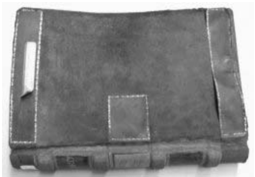
Fig 1. Effect of changes in temperature and humidity (Leather bound book warped and suffering from "Red Rot"). (Source: http://dlis.dos.state.fl.us/archives/preservation/books/index.cfm )
