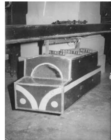
Fig.3 Single Primary Double Secondary LIM (fitted with bearings for movement and lateral guidance of OH transport system) [1972, 1983]
