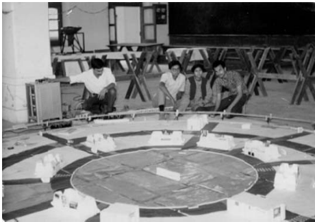
Fig 8 LIM Powered People Mover system for closed-loop circular track for Connaught Place people transport system
